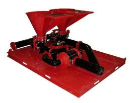
Single-shear hopper units excel at hydrating/suspending water- and oil-base mud products to ensure full yield of the product at addition, rather than circulating to achieve the desired rheological properties of the fluid. The addition of products and pre-hydrated mud from surface to TD is optimized, and unhydrated product is eliminated at the bottom of tanks to reduce product consumption and decrease pit, shaker, and basket strainer cleanout times.
